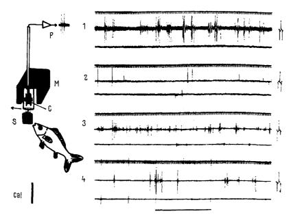
As illustrated in the diagram at the left, fish touching and striking at the gauze sack (S) produce small potentials across the coil (C) when this moves through the magnetic field of the magnet (M). Potentials so produced are amplified and recorded by a penwriter (P).
